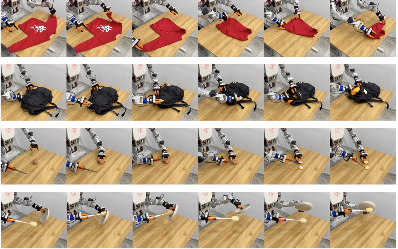
Fig. 4: Snapshots from teleoperation demonstrations on OpenPyRo-A1. Tasks demonstrated are (from top-row to bottom): (i) fold clothes, (ii) open bag and pick out item, (iii) slice the apple, and (iv) wash the dish.
